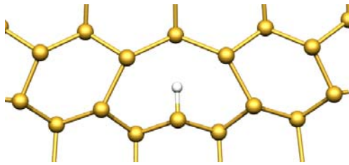
Fig. 3. Hydrogenated soliton defect in the dislocation core.
